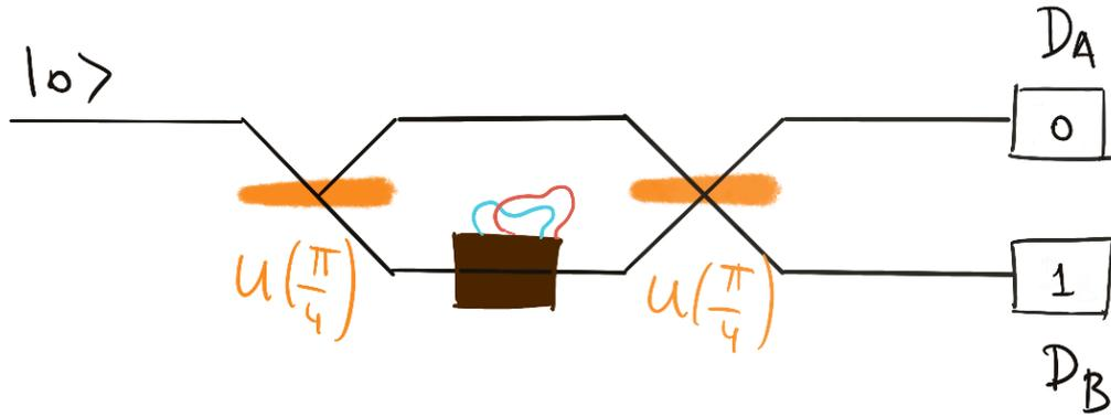
Figure 1: The experimental setup of Elitzur-Vaidman bomb tester.
