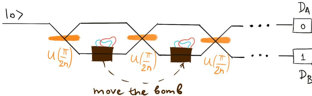
Figure 2: The experimental setup of Elitzur-Vaidman bomb tester with  $n$  copies of beam splitter (after each step we move the box further along the interferometer).
